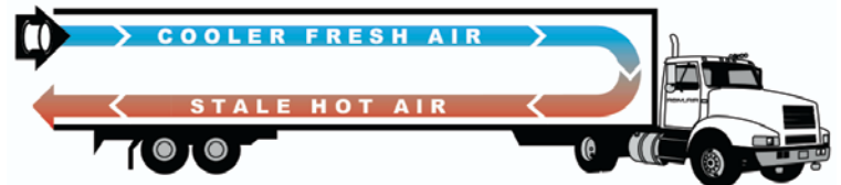
High-Velocity Air Circulator in a Truck Trailer
