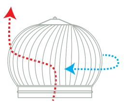
Spinning turbine head draws hot air out of the building.
