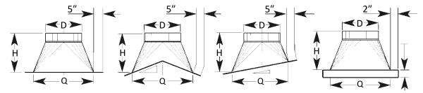
Base type and roof pitch must be specified when ordering (i.e. B-12 ridge 4" in 12" pitch)
